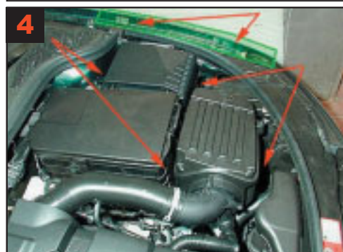
Front wing/wheel arch liner: Treat via existing holes and gaps.
