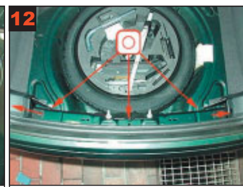
Rear panel: Remove plastic plate for correct treatment of panel.
