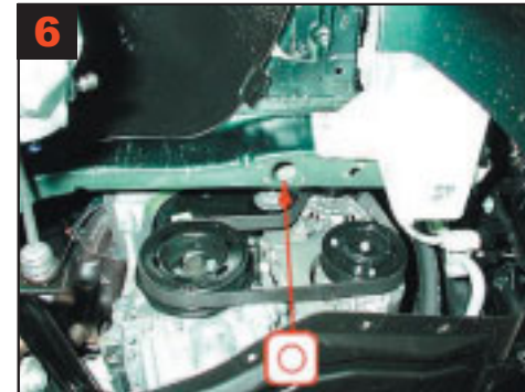
6 Wheel arch front/longitudinal member: Treat via existing hole.
