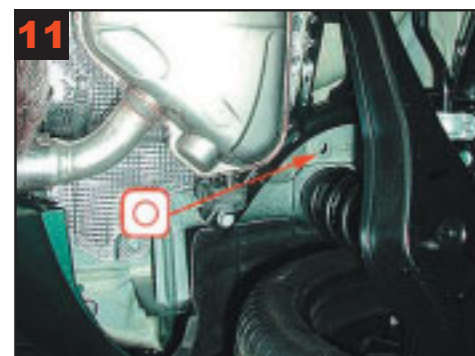
11 Longitudinal members in wheel arch rear: Treat via existing holes.
