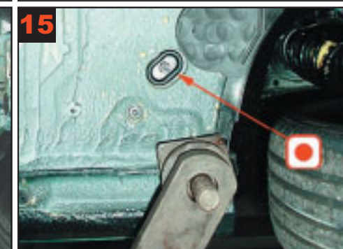
15 Small cross member after front wheel arch: Treat via existing plugged hole.
